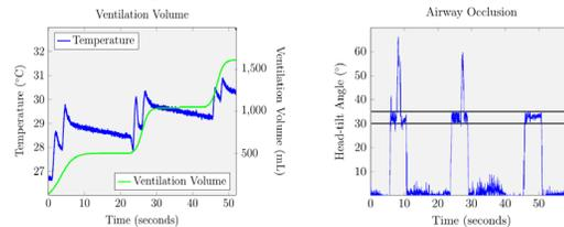
Figure 6. The thick blue line indicates the temperature measured by the manikin's thermistor, while the thin green line indicates the ventilation volume delivered, approximated from the temperature changes.
