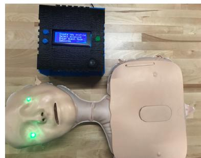
Figure 10. The fully operational manikin is displayed with all sensor equipment hidden under the mask and chest cavity. The enclosure above the manikin hosts the Arduino, LCD, and function selection buttons.
